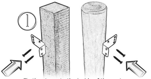
Fix the straps to the inside of the posts, we recommend a minimum of 6 straps per 1.8m panel & using number 8 (4mm diameter shank) countersunk screws 40mm long
